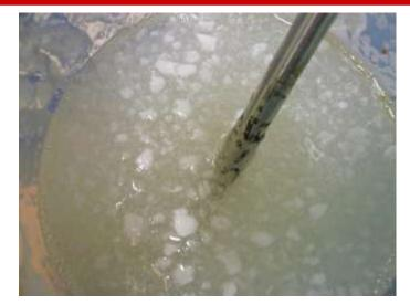
Couplant <u>not</u> specific for Ultrasonic Testing (example: glue, grease, oil...)
