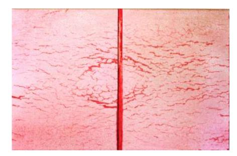
Red Penetrant Elite K71HT, White Developer D200 and Remover/Cleaner RHT are qualified <u>10° to +200°C</u>
