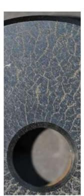
Cracks on pipe shown at +120°C (+248°F) with dualresponse fluorescent magnetic powder Elite FW1AC concentrate for water dilution
