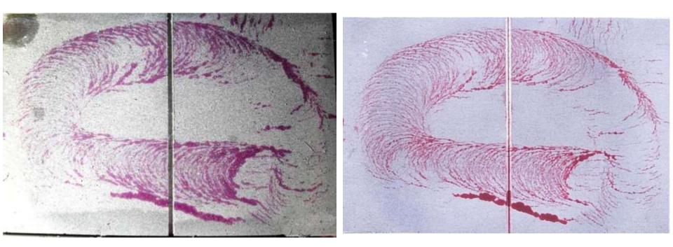
Red Penetrant Elite K71B2p, White Developer D112A and Bio Remover/Cleaner BC1 are qualified <u>-10° to +100°C</u>
