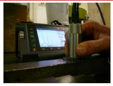
Couplant <u>specific</u> for Ultrasonic Testing
