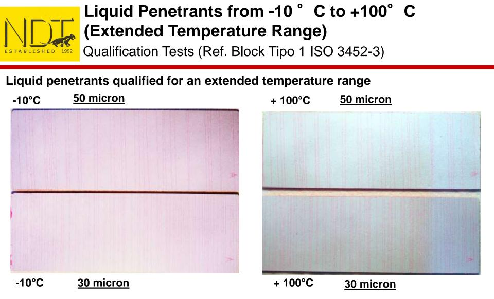
Red Penetrant Elite K71B2p, White Developer D112A and Bio Remover/Cleaner BC1 are qualified <u>-10° to +100°C</u> (tested according to ISO 3452-5 and ISO 3452-6)
